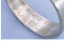
• Scuffing on inner ring bore surface of Tapered Roller Bearing
