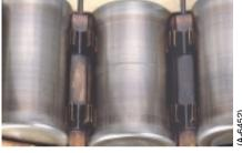
■ Scratch on outer ring raceway surface of Double-Row Cylindrical Roller Bearing Roller which slides when running.
