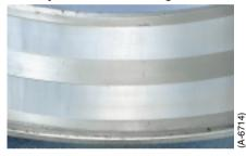
• Fretting on inner ring bore surface of Tapered Roller Bearing
