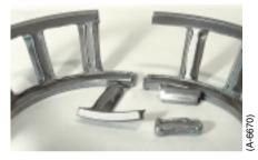
• Distortion of Cylindrical Roller Bearing cage
