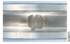
■ Flaking on inner ring of Cylindrical Roller Bearing
