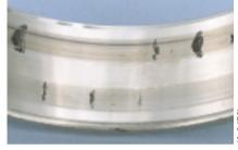
■ Rust on roller rolling surface of Cylindrical Roller Bearing
