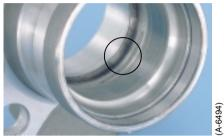
■ Rust on outer ring raceway surface of Double-Row Cylindrical Roller Bearing
