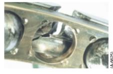
■ Crack in outer ring of Double-Row Cylindrical Roller Bearing
