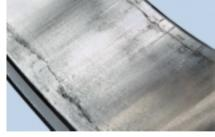
• Scuffing on inner ring rib face and roller and face of Cylindrical Roller Bearing with rib
