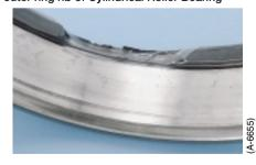
• Chip in outer ring rib of Cylindrical Roller Bearing
