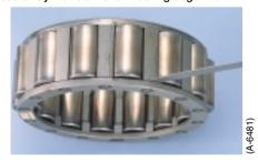
• Rust on Tapered Roller bearing cage
