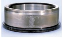
■ Flaking on outer ring of Double-Row Cylindrical Roller Bearing
